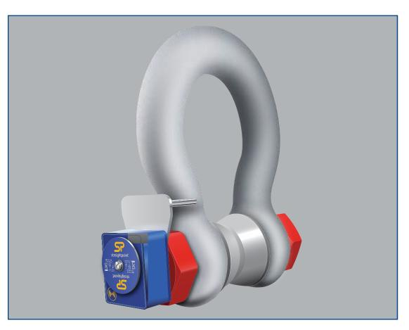
Available from stock in capacities 3.25t to 120t and available up to 1,550t, the WLS is manufactured from Crosby's industry leading 2130 Carbon and 2140 Alloy Bolt Type Anchor Shackles (3.25te - 120te) and the GN H10 Alloy Bolt Type Anchor Shackle (200te on up).
