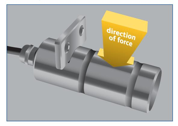
The Straightpoint range of Load Measurement Pins (LMP's) are designed for use in custom or bestspoke applications where more common, traditional load cells are not applicable. Load pins commonly replace for example, Sheave pins and and Clevise pins to provide an integrated solution.
