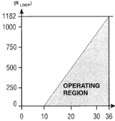
$$V_{min} = 10V + (.022A \times R_L)$$
