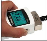
The Plug & Test<sup>TM</sup> connector locks into the receptacle in the indicator when fully inserted. Dual buttons on the indicator housing release the connector for easy removal. Gold plated spring contacts ensure long llasting and reliable connection
