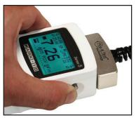
The Plug & TestTM connector locks into the receptacle in the indicator when fully inserted. Dual buttons on the indicator housing release the connector for easy removal. Gold plated spring contacts ensure long llasting and reliable connection.
