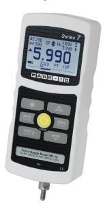
Thank you for purchasing a Mark-10 Series 7 digital force gauge, designed for tension and compression testing applications from 0.12 lb to 1,000 lb (0.5 N to 5,000 N) full scale. The Series 7 is an essential component of a force testing system, typically also comprising a test stand, grips, and data collection software.
