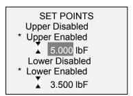
Either one, two, or none of the set points may be enabled. To toggle between the tension and compression directions, press the **DIRECTION** key.
