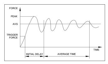
Average mode is used to obtain an average force reading over a specified period of time. This reading also represents the kinetic coefficient of friction, if the COF unit is selected. Applications include measurement of peel force, COF, muscle strength, frictional force, and other tests requiring time-averaged readings.
