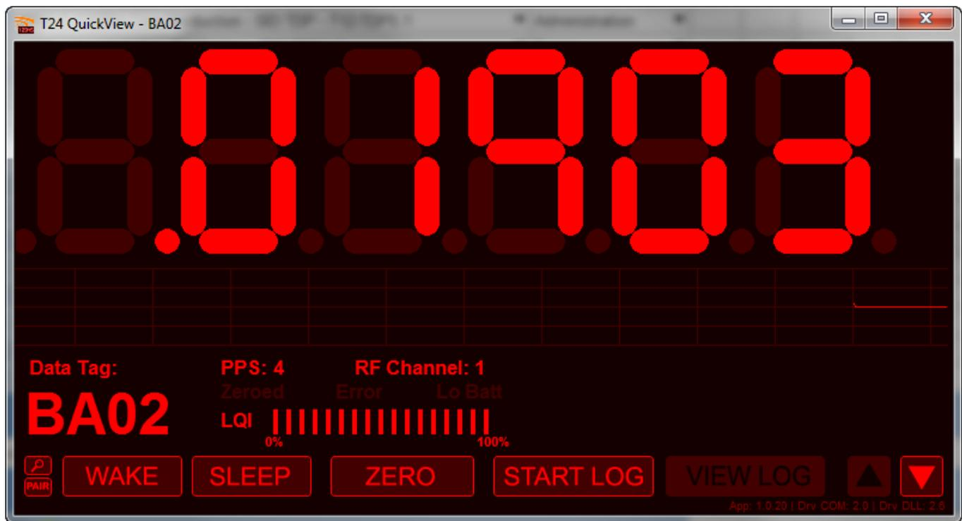
The software allows for a remote "wake" or "sleep" of the MasterLink 3000 amplifier to preserve battery power. A .csv log file is also generated through the "Start Log" command. This .csv file can then be opened in a spreadsheet program for graphing and other analysis. Battery power and signal integrity can also be monitored utilizing this tool.
