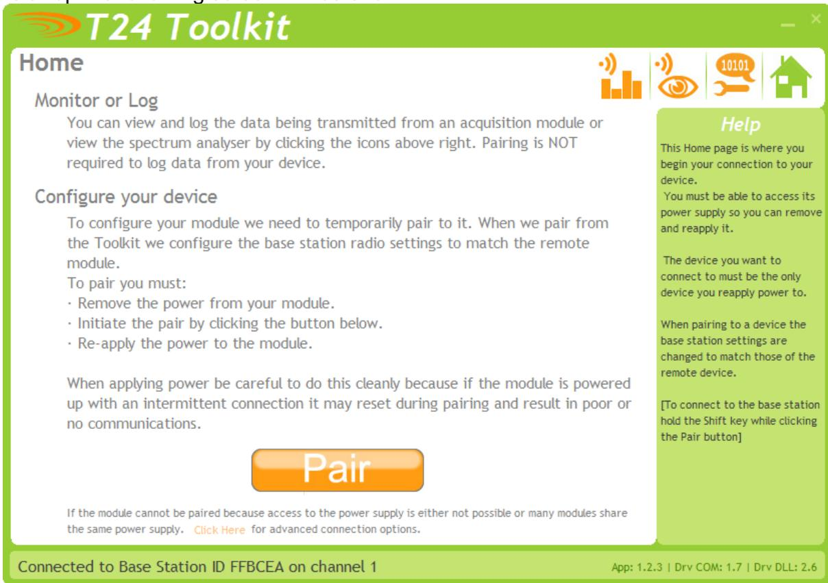
The "Pair" button is used to link the MasterLink 3000 amplifier, the MasterLink 3000 Handheld, and the MasterLink Analog Output to the MasterLink 3000 USB module. This is a one-time step necessary to configure the relative device.
