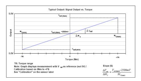
$V_{out(max)}$  and  $V_{out(min)}$  are defined with the slope of the sensor. i.e. the output voltage could be between 0.5 V and 4.5 V. The actual signal output range depends however on the calibration value.
