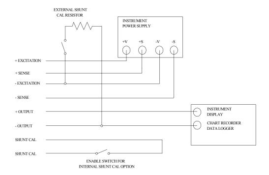
I. EXCITATION: The voltage being supplied to the transducer across the excitation terminals.
