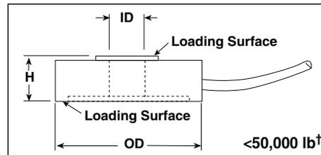
† Units >50,000 lb top and bottom loading surfaces are through the center hub.
