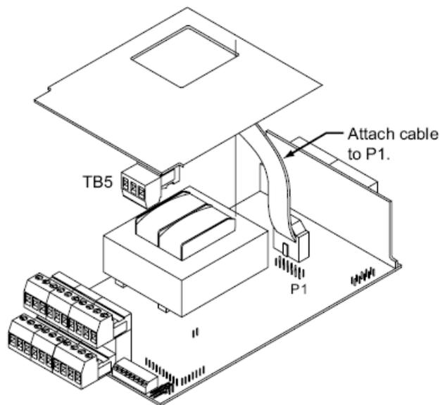
Figure 3-3 Upper Isolated Analog Output Option Board Installation
