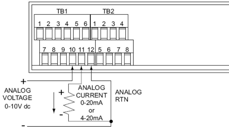
Figure 3-14 Analog Output Connections
