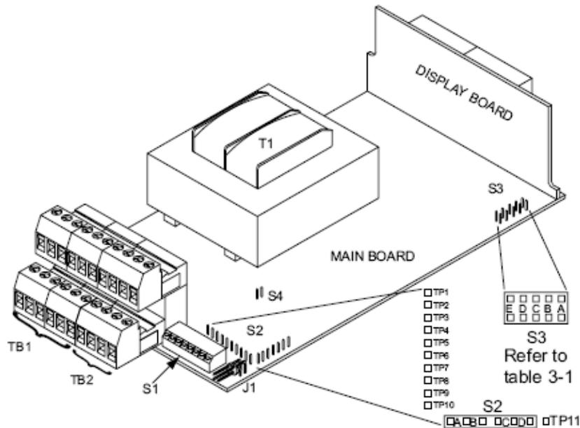
Figure 3-2 Main Board Jumper Positions
