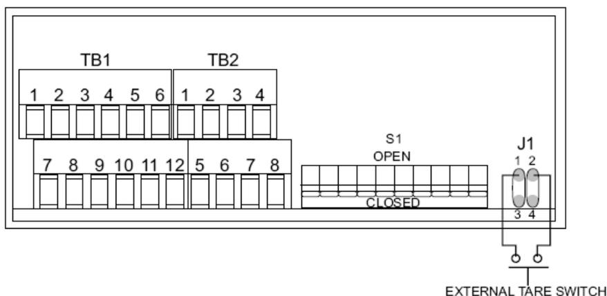
**Figure 3-13 External Tare Connections**
