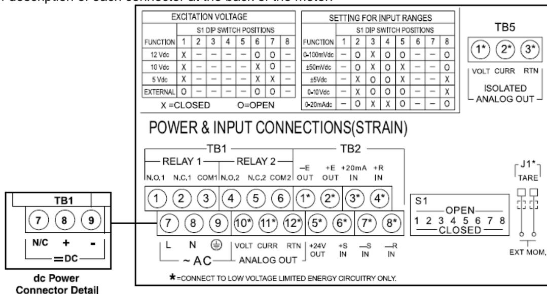
Figure 2-3 Connectors (AC-Powered and DC-Powered Detail)
