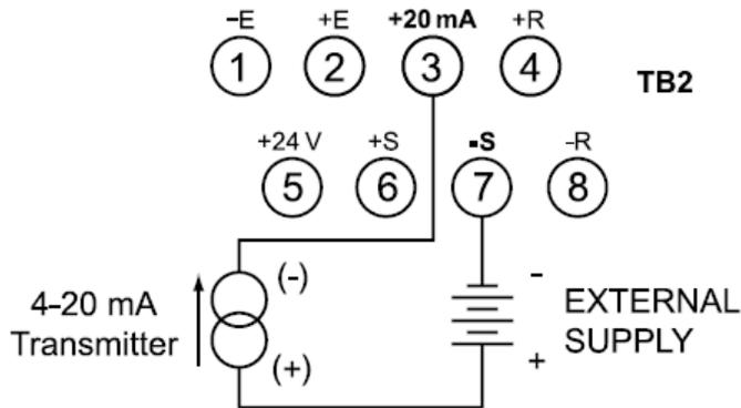
Figure 3-10 Current Input Connections with External Excitation
