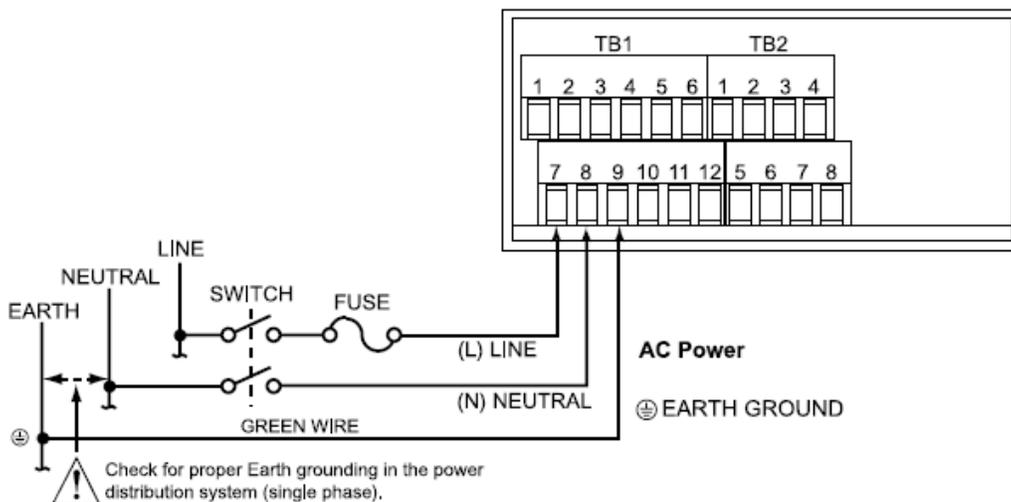
Figure 3-11 Main Power Connections - AC
