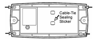
Affix sealing stickers to the rear of the instrument, over one or more screws in the locations indicated. Also affix a sealing sticker over the load cell cable where the cable-tie strain relief is attached, as indicated.
