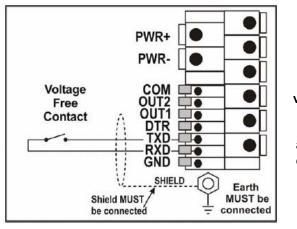
WARNING The remote input is a voltage free contact (e.g. button, mechanical relay). Connection of any active circuitry may damage the instrument.
