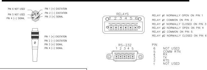
THE ABOVE DIAGRAM DEPICTS THE WIRING FROM THE CABLE ASSEMBLY OF THE LOAD CELL TO THE CONNECTOR FOR THE METER
