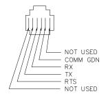
THE ABOVE DIAGRAM DEPICTS THE WIRING FROM THE CABLE ASSEMBLY OF THE LOAD CELL TO THE CONNECTOR FOR THE METER
